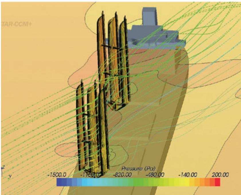
Lloyd's Register CFD images while wind testing a Windship rig fitted ship with two rigs
