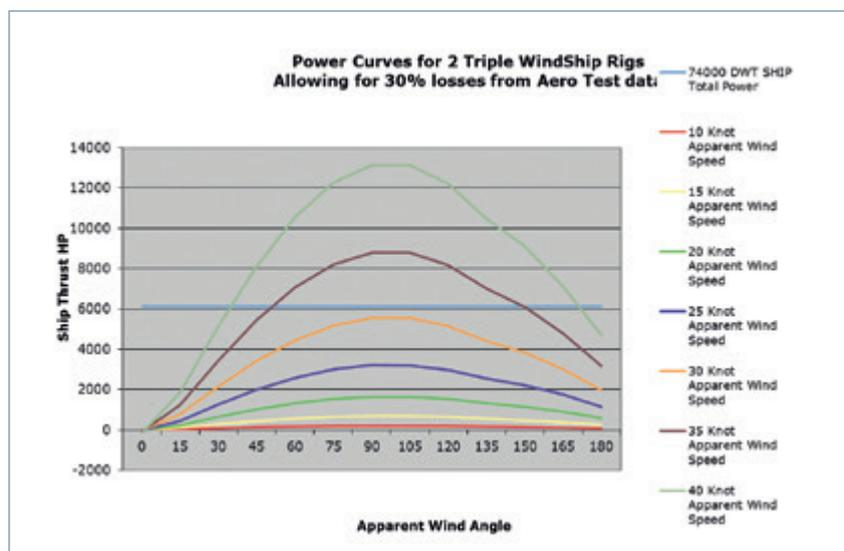
6,000hp is the normal thrust of an engine – the power curves show how much power can be generated using the wind and Windship rigs
